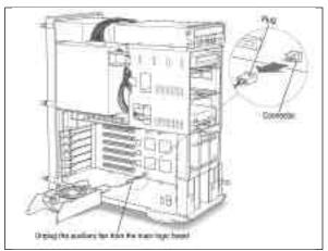
Unplugging the auxiliary fan (retaining clip on 8500)
